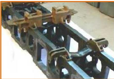
The photo on the left shows the casting made to represent mainly the mid boiler supports and the valve gear reverse shaft. Also shown are the main driver brake hanger support castings.
